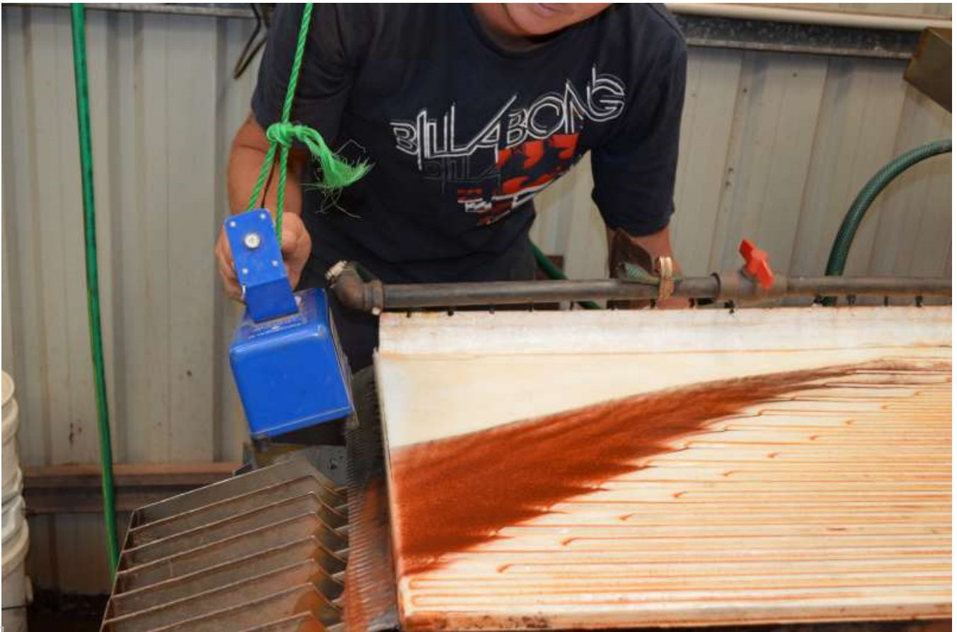
Photograph 1: Using UV light to check for Scheelite in the tabling process
